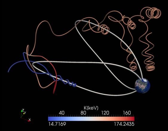
3D particle simulation of an O<sup>+</sup> ion subjected to a dipolarization front. Kinetic energy increases from 15 keV to 175 keV as the O<sup>+</sup> "bounces" against the incoming front. Protons (not shown) are energized too but not as effectively.
