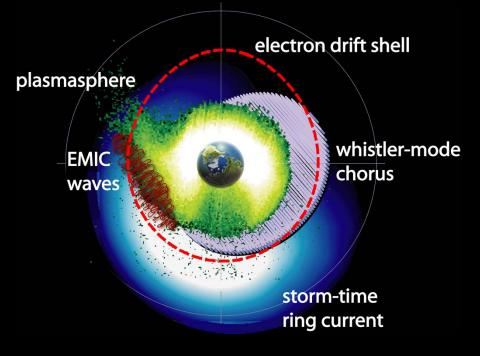
The variability of the outer electron radiation belts are due to competing global and local acceleration and loss processes, such as chorus waves and ULF waves versus magnetopause shadowing and EMIC waves.
