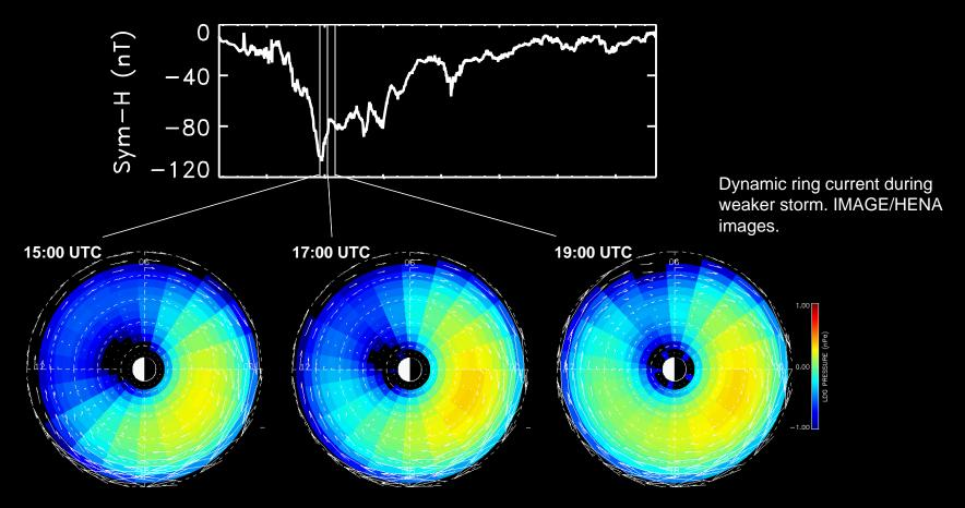
Global ENA images show that the ring current changes from highly asymmetric to symmetric in a several hours only. The plasma proton pressure derived from images in the 60-119 keV range shown. The ring current can also be highly symmetric in the storm recovery phase depending on IMF.
