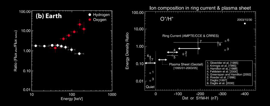
**Left**: ratio of post- and pre-substorm flux of O and H demonstrating mass dependent acceleration *[Keika et al., 2010]*.
